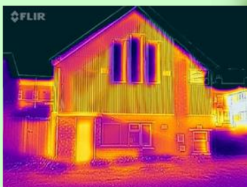
St Nicholas' showing heat loss through the roof, internal, and South side, external.
